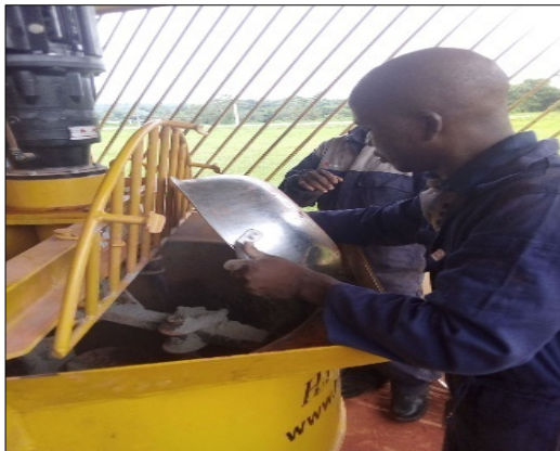
Fig 7: Pouring waste brick material into hydrofoam brick making machine
