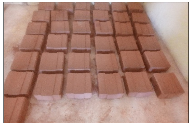
Fig 9: Air curing of produced bricks
