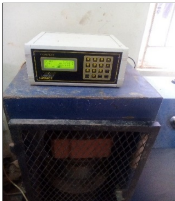
Fig 5: Compressive strength test of brick
